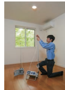
Inspection for VOC concentrations and allergens in a newly built home. This practice has led to the eco-friendly Airkis , our high-quality indoor air system.
